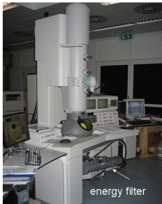
Figure 3.9 Transmission electron microscope equipped with GATAN energy filter at MESA + .
